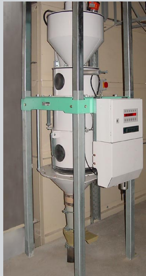
Transflowtron Scale in a flour mill.
