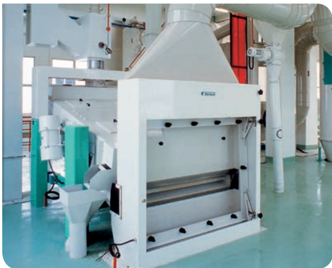
Separator MTRC – efficient sorting and classifying machine.
